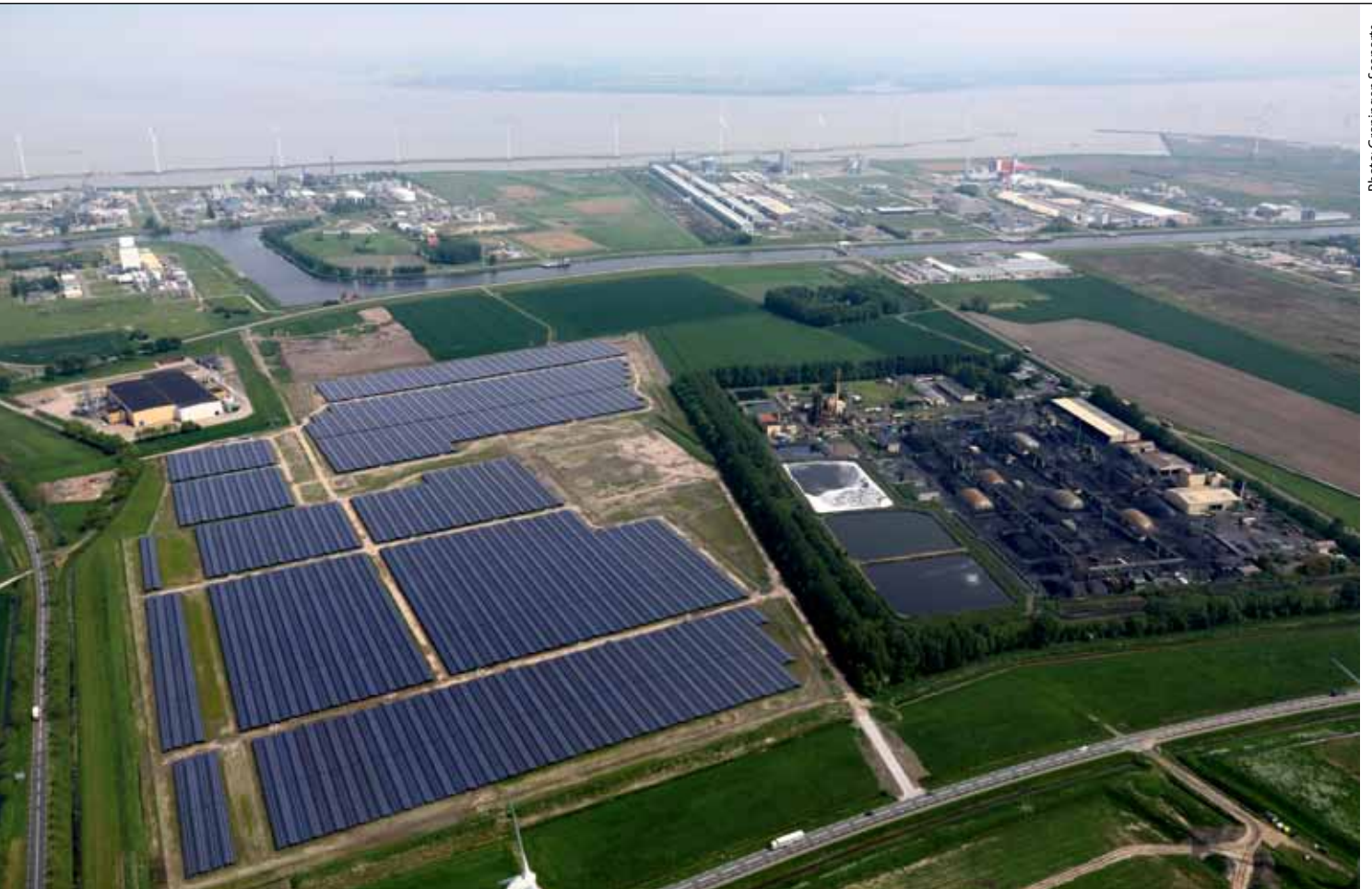
The 30 MW Sunport Delfzijl is currently the Netherlands' largest PV project, powering a Google data center in nearby Eemshaven.
